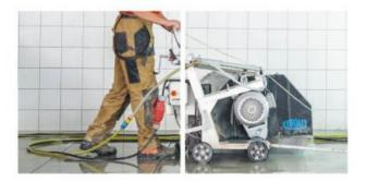
Diamond cutting eliminates vibrations and reduces concrete jackhammering noise. Thanks to the use of wireless saw control, the risk of injury to operators is reduced.
